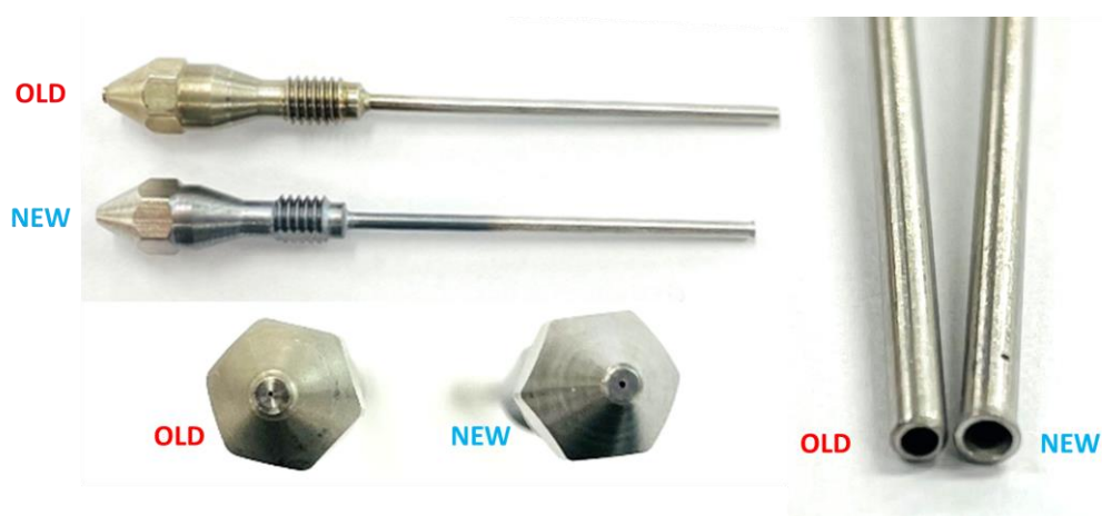
Figure 1. Capillary Jet for FID Detector (Old & New)
