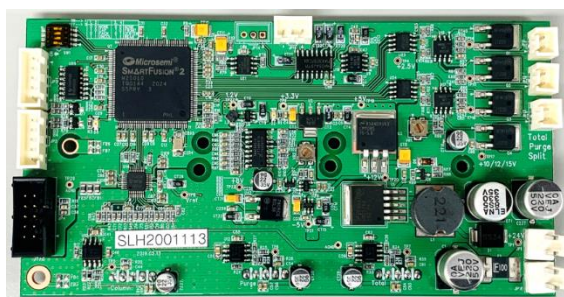
Figure 1. UPC Inlet Board for ChroZen GC (P/N 6701538110)
