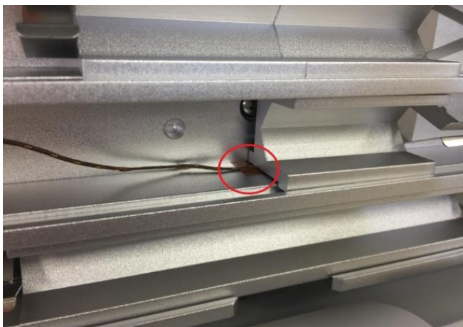
Figure 2. Probe position in the heating block -2
