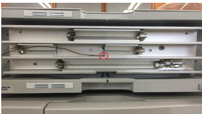
Figure 1. Probe position in the heating block -1
