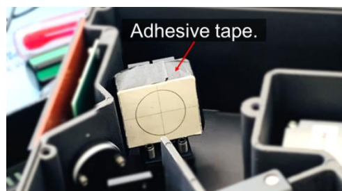
Figure 6. Put the test jig on the center of the grating.
