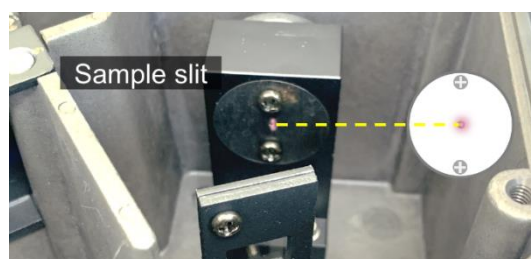
Figure 14. The exact position of the light beam on the sample focus slit.
