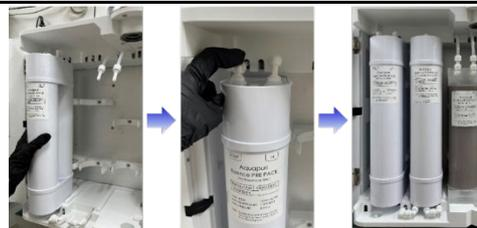
5. After filter replacement, press **[Select]** to flush filters for 30 counts. After filter flushing, the filter usage time will be initialized.
